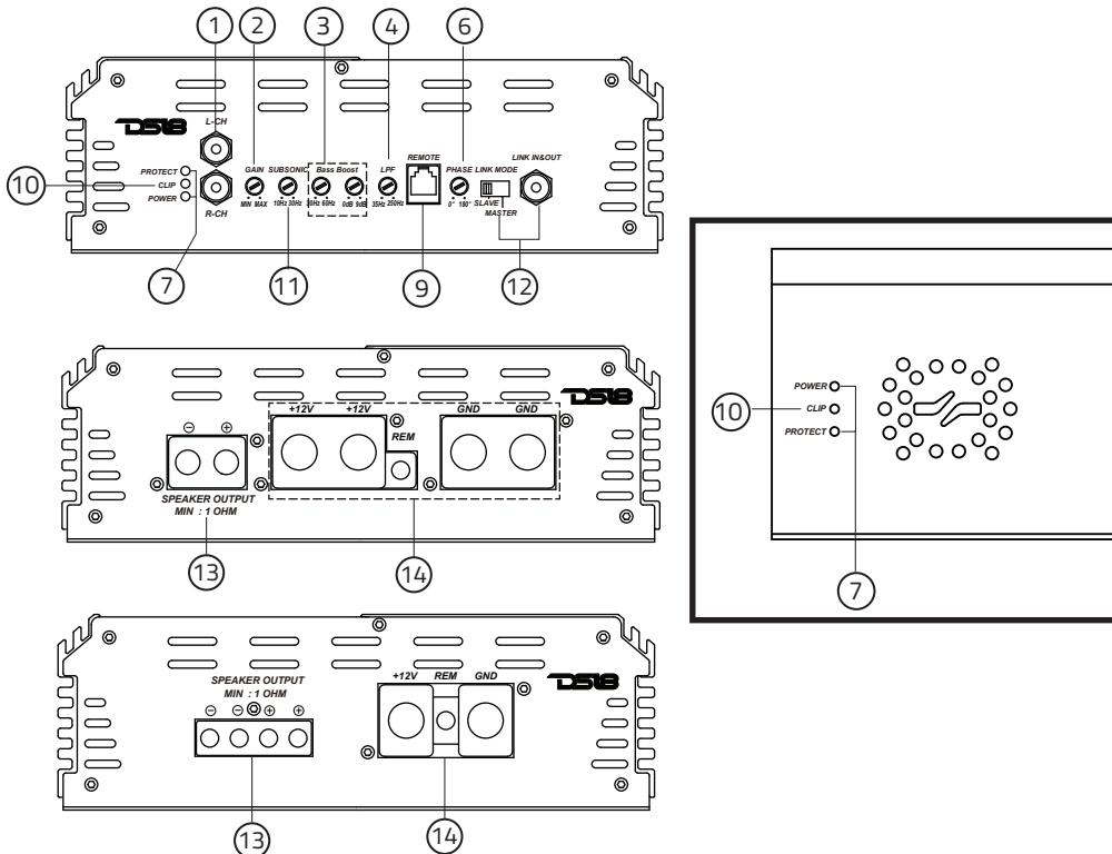
**1. RCA AUDIO INPUT CONNECTION** - Using high-quality shielded stereo RCA cables, connect the source signal to the amplifier RCA inputs.
