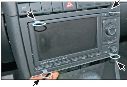
2. Use 4 radio release keys to dismount the OEM radio.
