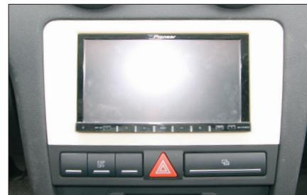
5. Connect alle required circuit points and push the double DIN head unit until it snaps in.
