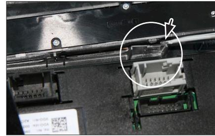
5. Unclip and remove switch panel below air condition control unit
