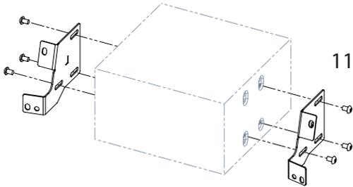
11. Attach mounting brackets to double DIN navigation
