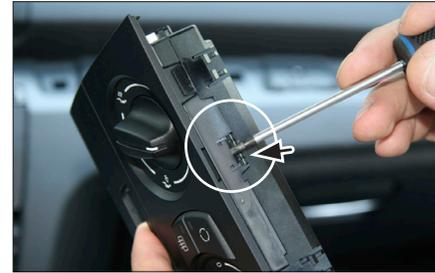
6. Unclip and remove air condition control unit
