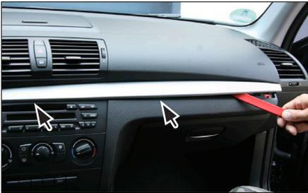
2. Unclip middle panel and remove it carefully
