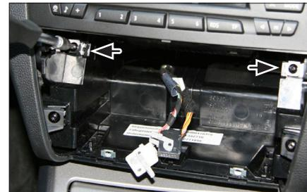
7. Remove screws below OEM head unit (see arrows)
