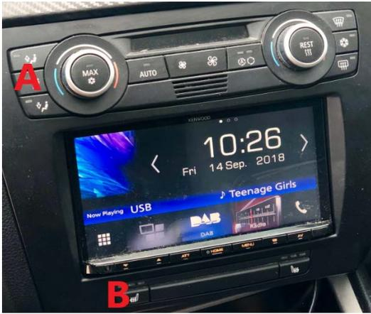
10. Attach air condition control unit (a) and switch bar (b) to replacement facia plate
