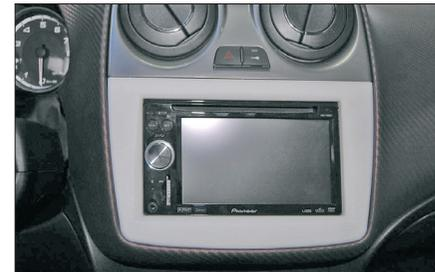
5. Push the Metal Frame into the facia plate, place both into the dashboard.
