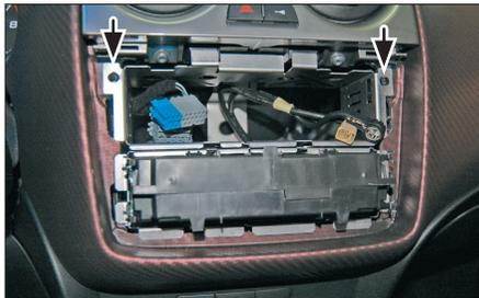
3. Remove the original metal holder inside the the dashboard, which is fixed by 2 screws (see arrows)
