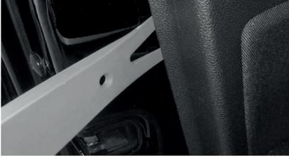
When the door panel is loose, start by softly lifting the panel straight up to remove it.
