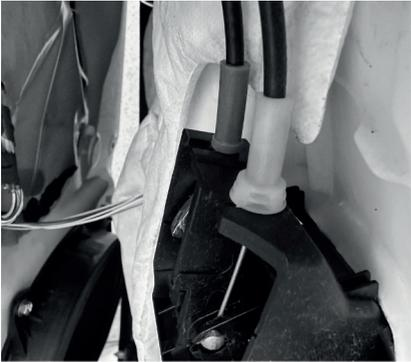
Disconnect electrical connections for the door lights.
