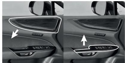
In most cases the screws used are Phillips type, use a tool bit PH2 size. Unscrew them and store the screws in a safe place, for later use when reinstalling the door panel.
