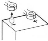
Place the disconnected terminal in a secure and isolated location away from any possible connection belonging to the battery/power source system.
