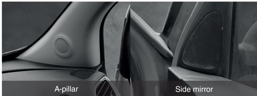
Start by removing the tweeter covers. Use plastic pry tools and be careful, there can be air-bags behind the A-pillar. The first clip can be hard to remove. Take it easy and use minimal force. The instructions below shows how to remove the A-pillar tweeter.
