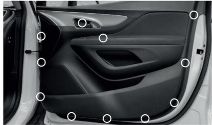
Usually the clips/screws are placed by the white marks. This could vary depending on the vehicle.
